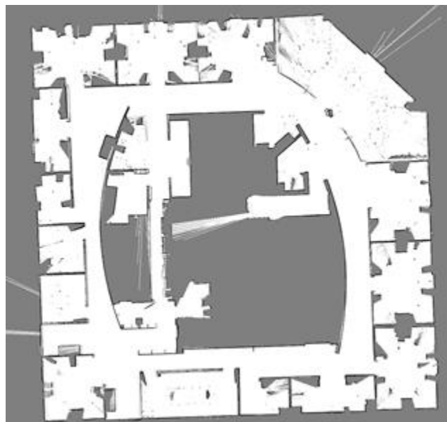
Figure 3.2: Intricate SLAM Map showing spikes and edges (Request Pending by SLAM for Dummies)
